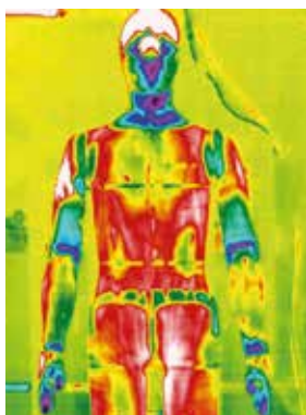
Standard SMS material Sweating Mannequin Test (35°C / 95°F; 30% fuktighet, 1 timme) Oberoende Lab Test – TPACC Lab, North Carolina State University
